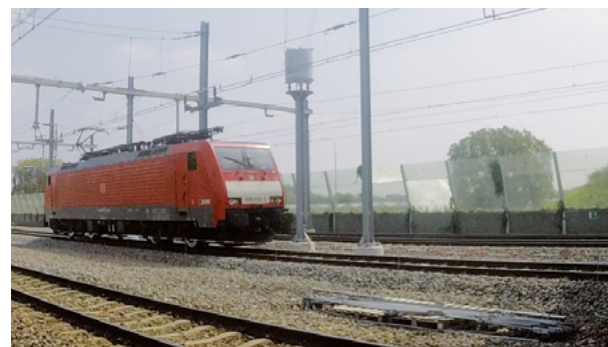
Fig. 4: Train ride in the system separation section, approaching from Emmerich (source: ProRail)
