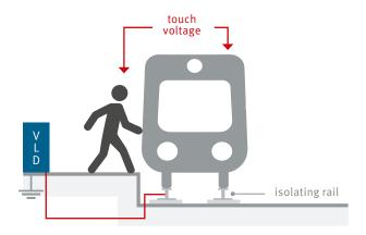
Protection and control with TracFeed® DCP3L
